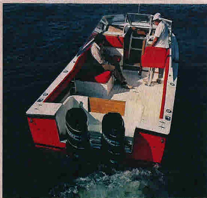
Above: Outboard boat with standard pedestal helmsman's seat and optional lounge-and-ice chest combination ($350). Cuddy cabin encloses V-berths and space for optional head. Right: Full-depth self-bailing motor well is fitted with teakwood gate for access to engines.
