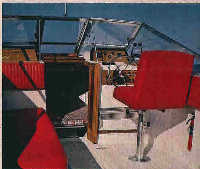
Above: Outboard boat with standard pedestal helmsman's seat and optional lounge-and-ice chest combination ($350). Cuddy cabin encloses V-berths and space for optional head. Right: Full-depth self-bailing motor well is fitted with teakwood gate for access to engines.
