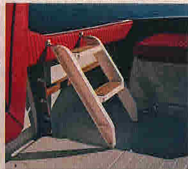
Left: Transom configuration marks the basic difference between the boats. Below: Mayfair Products folding, floating ladder doubles as cockpit ladder and access steps to nonslip foredeck through opening center panel of windshield.
