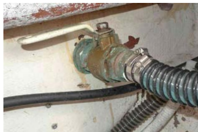
1.5" livewell overflow ball valve changed 2012, new hoses & AWAB clamps.
